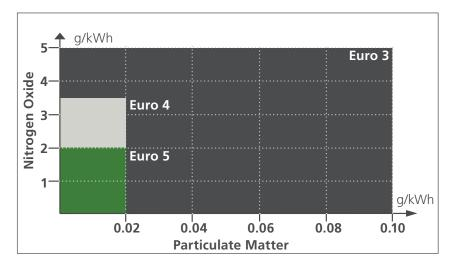
We vow to play our part for cleaner air that allows a sustainable environment for everyone. With Euro 5 SCR, nitrogen emissions are 43% lower and particulate matter emissions are 80% lower than Euro 3 levels. Compared with Euro 4 levels, Nitrogen oxides are 43% less.
