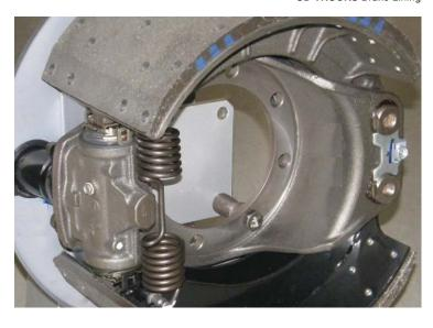
UD Brake Drums are designed and manufactured to be exactly round with zero tolerance. They have a unique profile that allows uniform thermal expansion. The force created when braking means that the brake drum must absorb high levels of energy. Temperatures created by the contact between the drum and the linings can be as much as 500°C.
