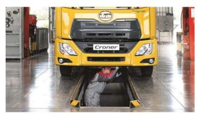
You can depend on Genuine UD Service when it comes to installing replacement parts on your truck. Brakes should be replaced in pairs to secure brake system efficiency and safety.
